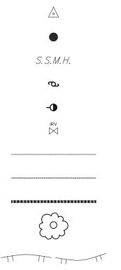
RANDOM CONTROL FOR FOUND MONUMENT AS i SANITARY SEWER MANH EXISTING POWER POLE EXISTING GUY ANCHOR EXISTING IRRIGATION VA EXISTING WOODEN FENC EXISTING WOOD RAIL FE PROPERTY LINE
